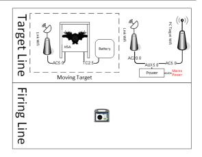
The PC Target antenna sets up a Wifi network covering 400 meters.
